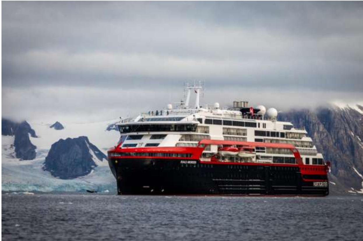
The Roald Amundsen above also has the signature large white globes used to protect the 5G antennas, two small ones near the front of the ship, and three larger globes toward the aft deck (only two are visible).
