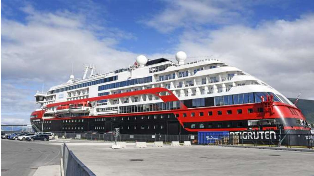
Hurtigruten's Roald Amundsen is an expedition cruise ship with a strengthened hull capable of driving into ice in the Arctic. The above picture shows clearly the two larger 5G white domes from the aft area. These large white domes are required to protect the 5G satellites from rain, snow, ice, sleet, dust, and fog from interfering with communications to the low and mid-level orbiting satellites.
