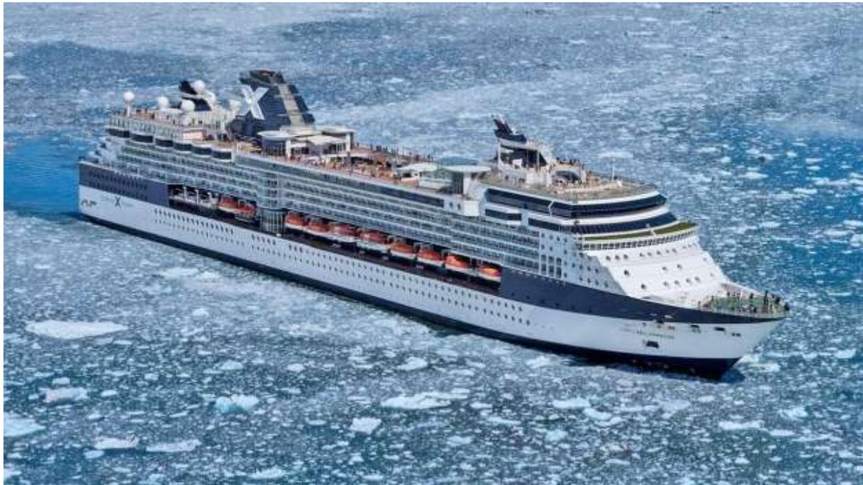
If you look closely in this  $\frac{3}{4}$  aerial view in Arctic waters, you can see the 5G white globes extending high above the aft area's 11<sup>th</sup> deck of the Celebrity Millennium. These globes protect the 5G antenna transceivers from the elements. 5G because of its use of millimeter wave spectrum requires an obstacle-free point-to-point line of wireless communication. 5G has an Achilles heel so to speak, it is vulnerable to fog, sea mist, snow, ice, rain, dust, and cloud cover.
