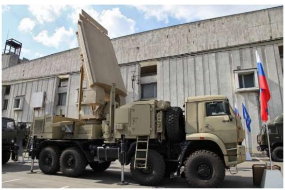
The radar unit above can command and control several different batteries of missiles and guns.
