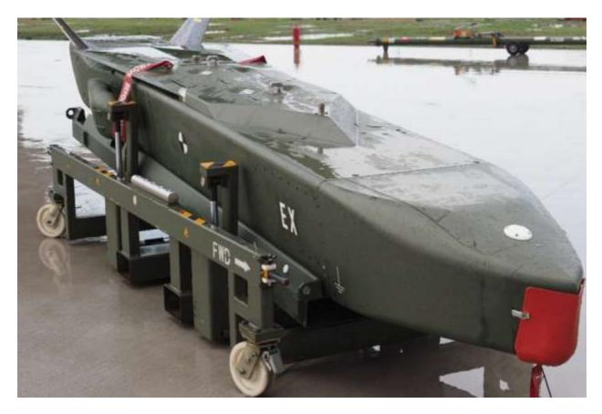
The dual stage 480-kilogram (1,100 lb.) warhead, called MEPHISTO (multi-effect penetrator highly sophisticated and target optimized), features a pre-charge and initial penetrating charge to clear soil or enter "hard and deeply buried targets" (HDBT) such as hardened underground bunkers, then a variable delay fuse to control detonation of the main warhead.
