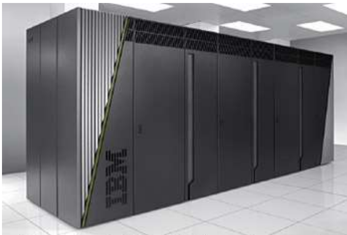
IBM Sequoia — As of June 2012 this computer became the world's fastest, surpassing one that had been developed by the Japanese. It operates at 16.3 petaflops, which means it can perform 16.3 quadrillion computations per second!
